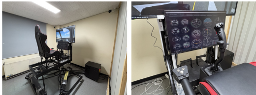
Fig. 2. 6-DOF motion simulator
