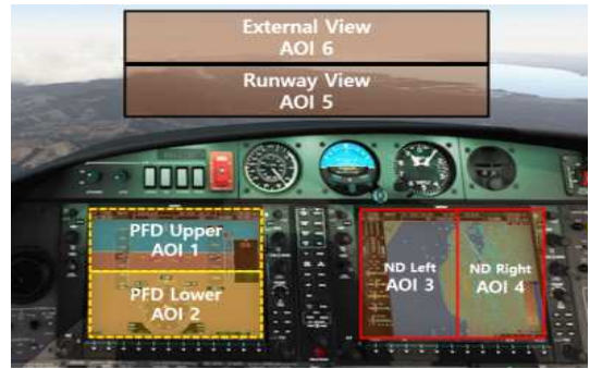
Fig. 10. AOI setup
