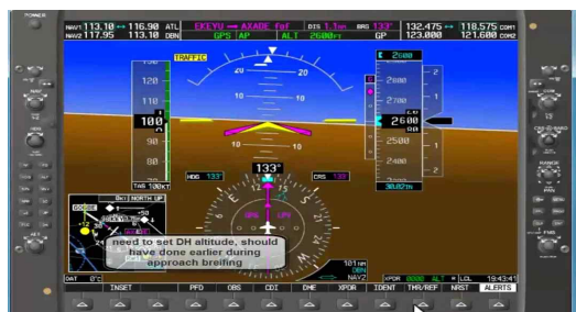
Fig. 4. G1000 digital cockpit PFD
